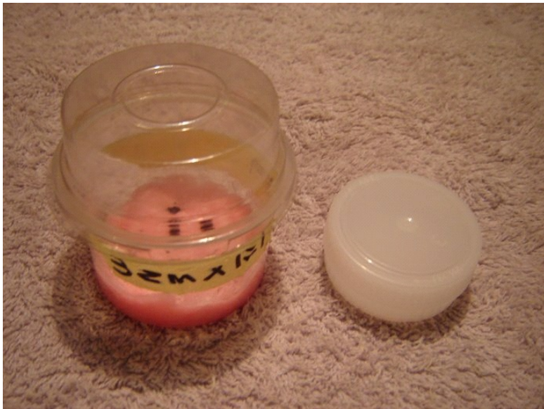
18/05/2010 - First Day - The container was sealed to keep moisture uniformly throughout the environment.
